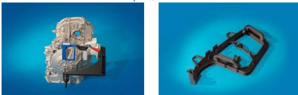
Figure 2 - Assembly lift assist, on the left, and window alignment tool, on the right, used by Ford in the assembly plants.
