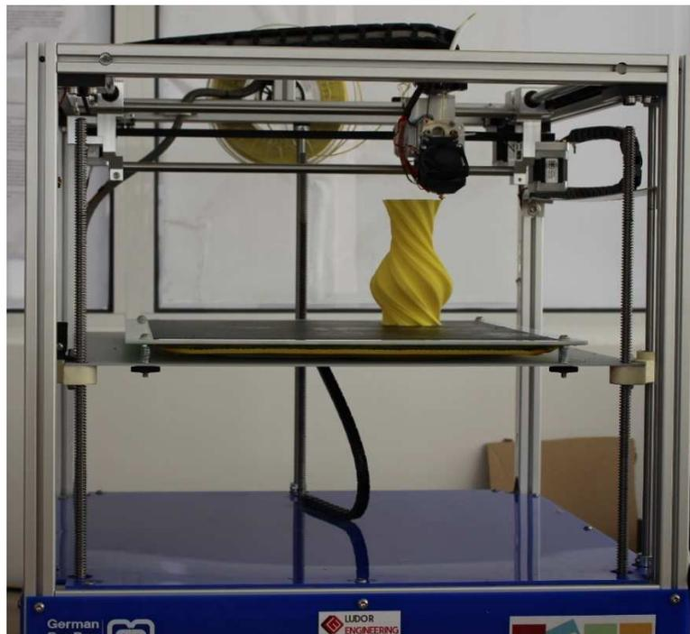
Figure 1 - FDM 3D printing. Fonte: Ludor Engineering
