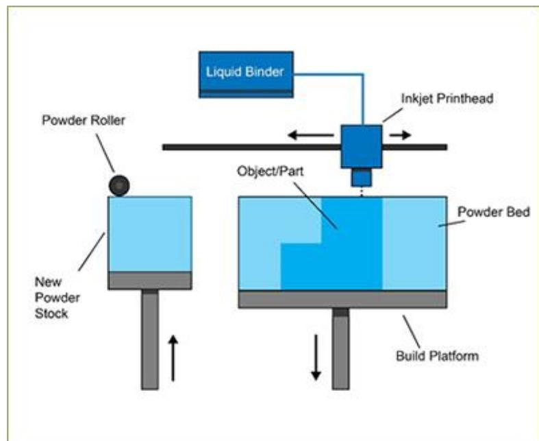
to be sintered to become fully metallic as the binding material is burnt. Typically, the printing head consists of multiple binder jets.
