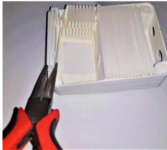
Figure 7 - Removal of the support structures
