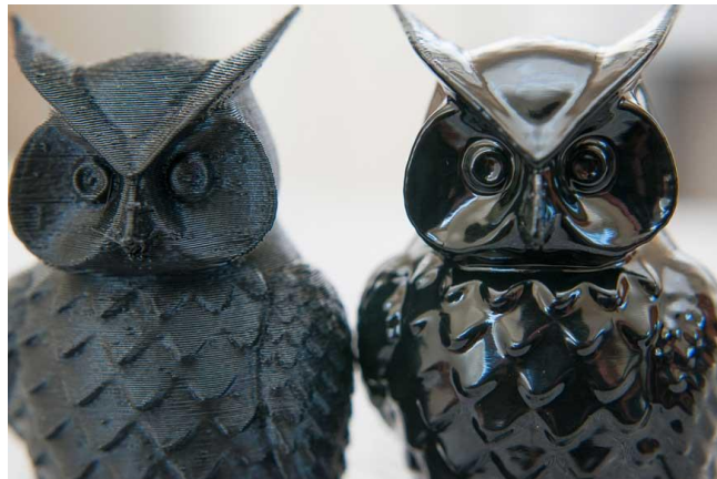
Figure 10 – A 3D printed object, before and after vapour smoothing. Source: www.qeetech.com
